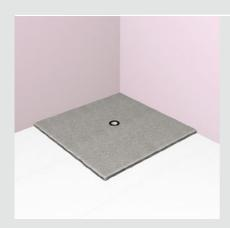
C Lay a level bed of fast-setting concrete around the trap to the size of the shower base, plus an extra 100mm in both directions, ensuring that the finished level is 32mm below the final floor level. Alternatively lay a pad of Beava Board, or similar cement faced tile backer board, to achieve the correct height. Beava Board is available in 7 thicknesses 5.5, 10, 12, 20, 30, 40 and 50mm (order separately).
