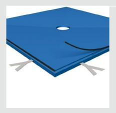
E Stick the temporary 6mm rubber strip into the rebate of the room-facing edges of the shower base.
