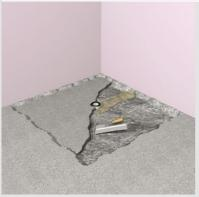
**B** Lay a level bed of fast-setting concrete into the whole cut-out area, ensuring that it is 32mm below the existing floor level.
