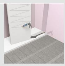
B Put trap and waste into position; the black rubber seal of the trap should be 28mm below the finished floor level, the trap may require recessing into the existing concrete floor. Put the trap and waste into position and fill round with a weak sand and cement mix.
