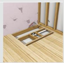
G Assemble and install the remaining parts of the trap, as specified in the instructions included in the trap box. Use the temporary plastic cover to protect the trap during tiling. Seal between the base and the wall with Mega Strength (the rebate against the wall will be filled with tile adhesive when tiling)
