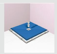
G When the screed is set, remove rubber protection strip and fill the gap with Mega Power, as well as gaps between the showerbase and the walls. If tiling over Kaskade, prime the surrounding concrete before tiling with two coats of SBR Tilers Primer, diluted 3:1, to fully waterproof it.
