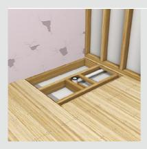
C Fix noggings or extra joists where required, to provide support to all edges of the shower base as well as closely around the outlet. Use Mega Strength adhesive to ensure a firm fix for noggings.
