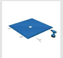
D Stick the temporary 6mm rubber strip into the rebate of the room-facing edges of the shower base.
