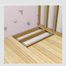
B Put trap and waste into position, and support with timber to the correct height; black rubber seal of the trap should be 22mm below existing floor level.
