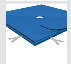
E Prime the concrete and then apply a bed of good quality flexible tile adhesive to the new concrete bed. Set the shower base on to the adhesive, ensuring that the top is flush with the existing floor level and that a 3mm gap is left between the shower base and the walls.
