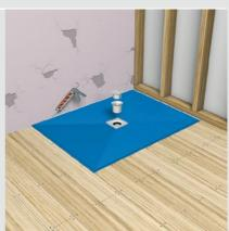
You can now overlay the floor with NO MORE PLY, overlapping the NO MORE PLY boards on to the rebated edge of the shower base, having first applied a good bead of Mega Strength to get a perfect seal. See separate installation instructions for fixing NO MORE PLY, or visit www.nomoreply.net
