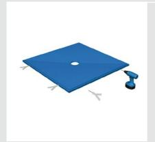
D Drill two 4mm holes into both outside edges of the shower base, and carefully screw in the four stainless steel anchors.
