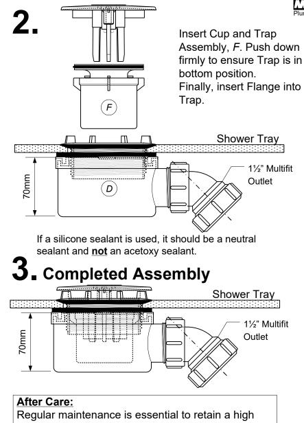
performance flow rate. Remove the Flange and Trap Assembly, *F*, and thoroughly clean all the parts. Flush through the Trap Body with clean water and carefully replace the parts.
