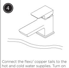
hot and cold water supplies. Turn on the mains water supply letting the water flow for a few minutes to flush through the system. Check all joints and connections for any leaks.
