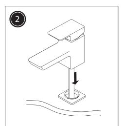
Place the plinth over the hole in the basin/ bath and feed the flexi tails through.
