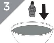
Place valves in a suitable solution and soak until fully de-scaled.
