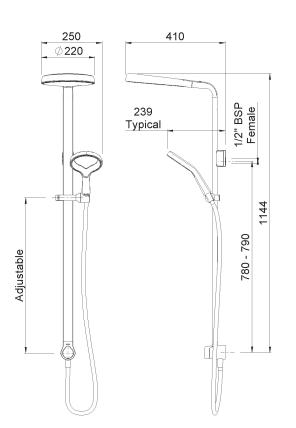
CONSTRUCTION: Brass & ABS CARTRIDGE/VALVE TYPE: N/A SUPPLY: Suitable for high pressure only INLET CONNECTIONS: 1/2" BSP WORKING PRESSURES: 1.0 - 5.0 bar
