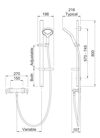
CONSTRUCTION: Brass & ABS SUPPLY: Suitable for high pressure only INLET CONNECTIONS: 15mm Compression WORKING PRESSURES: 1.0 - 5.0 bar CARTRIDGE/VALVE TYPE:Thermostatic
