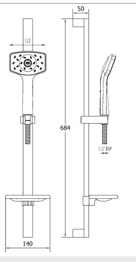
**CONSTRUCTION:** Stainless steel/ABS **SUPPLY:** Suitable for all plumbing systems
