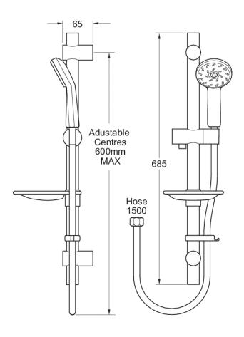
**CONSTRUCTION**: Stainless steel/ABS **SUPPLY:** Suitable for all plumbing systems
