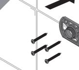
Secure the rubber backplate and backplate into place.
