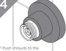
back of the wall outlet. securing them against the rubber fixing plate
